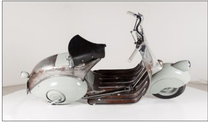
A Vespa from the 0 series, only 60 models were built in 1946. This model has a 98ccm one cylinder, two stroke, three-gear engine that is cooled by air flow. The vehicle shown here with the frame number 10031003 and the engine number 014 is the third Vespa ever built. As neither of the two previously built vehicles still exist, is this the oldest Vespa in the world. The market value of this roadworthy (!) vehicle: approximately 250,000 to 300,000 Euro.
