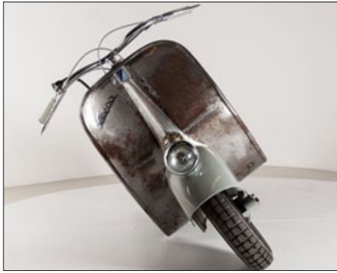
A Vespa from the 0 series, only 60 models were built in 1946. This model has a 98ccm one cylinder, two stroke, three-gear engine that is cooled by air flow. The vehicle shown here with the frame number 10031003 and the engine number 014 is the third Vespa ever built. As neither of the two previously built vehicles still exist, is this the oldest Vespa in the world. The market value of this roadworthy (!) vehicle: approximately 250,000 to 300,000 Euro.
